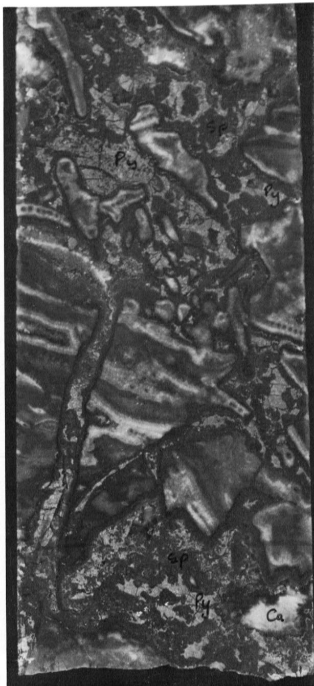
2a. Complex pyrite-sphalerite intergrowth in cavity. Cross-cutting fracture is sphalerite-lined with complex sulphide-fill. Note fracture cuts partially-sealed stromatolite cavities.
