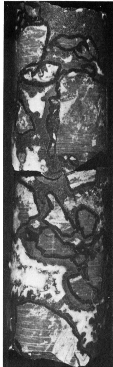
4c. Late fracture with pale sphalerite, cross-cutting sealed stromatactis. Fracture may itself have re-opened with two generations of calcite-fill. Note fracture terminates against a sub-horizontal stylolite.
