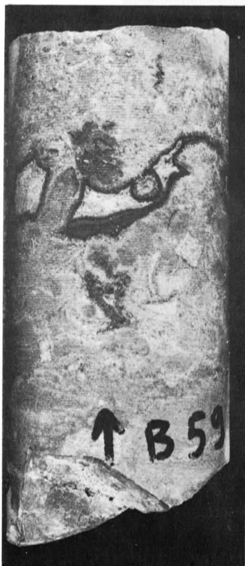
1c. Cavity-lining mineralization, alternating with geopetal sediment.
