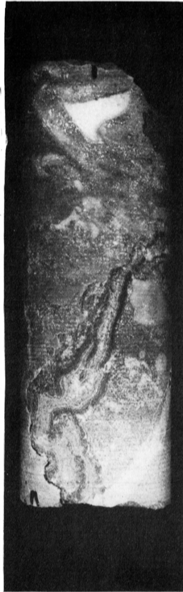
4b. Breccia mineralization. Sphalerite (dark grey) coating brecciated Waulsortian micrite.
