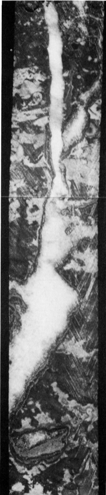
4a. Fracture or fissure lined with finely-laminated alterations of dark and light sphalerite. Note stylolitic contacts and crumpling of sphalerite laminae.
