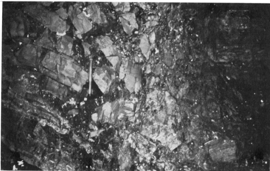
Figure 14. Photograph of the edge of a mineralized collapse breccia from the Gordonsville mine. Sphalerite (dark grey) fills open spaces between fragments of early fine-crystalline dolostone (light grey) derived from the hanging-wall of the breccia. Mottled beds in the lower left and upper right corners are equivalent units separated by reverse fault displacement along the side of the collapse breccia. The zone of displacement is occupied by mineralized breccia that dips from the upper left, down to the lower right.
