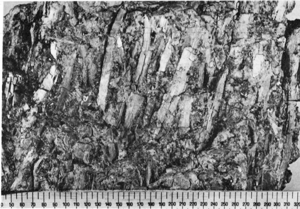
Figure 5. Spodumene pegmatite showing strongly aligned spodumene crystals in a matrix of quartz, mica and K-feldspar. Aclare House, Co. Carlow.
