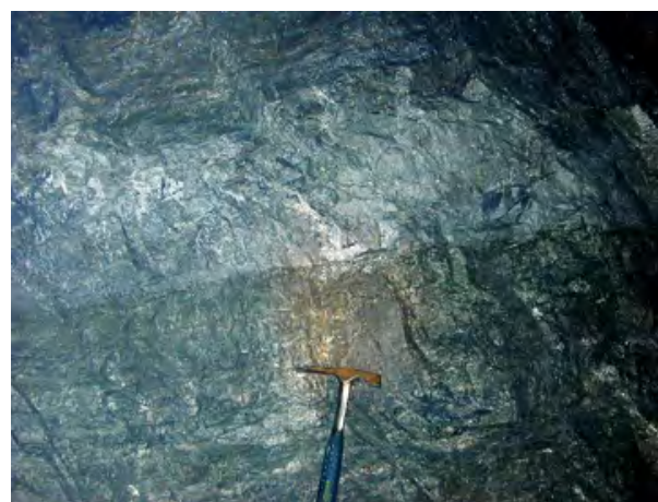
Figure 22: Banded sulphide, principally sphalerite and galena, developed by replacement of black matrix breccia. Within the breccia is a large slab of Waulsortian dolostone that is not replaced, (Main East, Lisheen).
