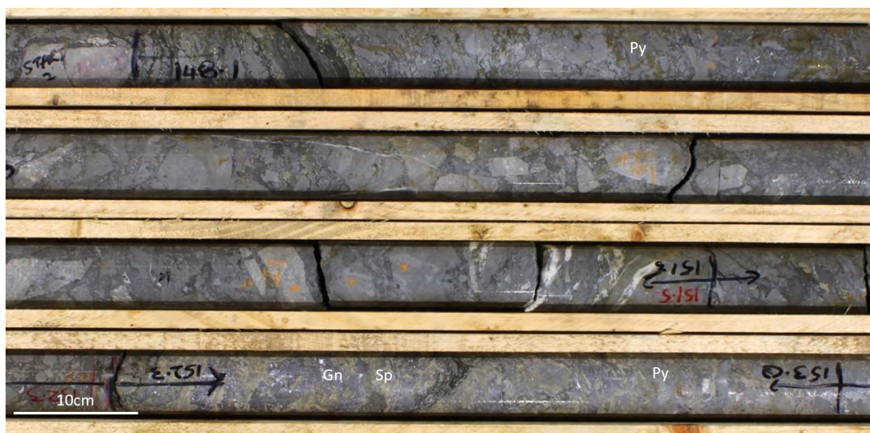
Figure 20: Black matrix breccia with various clast morphologies and minor pyrite (Py). The bottom run is significantly replaced by pale, tan-brown sphalerite, (Sp) and galena (Gn). From hole 4513-12, R-Zone, Galmoy.
