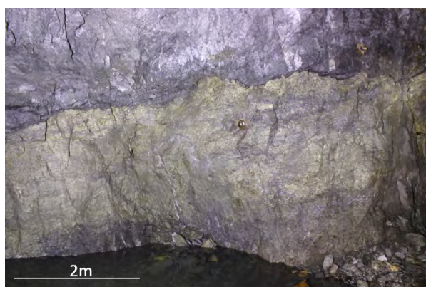
Figure 16: Sharp hanging-wall contact between pyritic massive sulphide and black matrix breccia above (Main North, Lisheen). Some pressure solution has occurred but is not considered to be significant. Sharp hanging-wall contacts are a feature of many massive pyritic bodies and bands. Very often the contact is with Waulsortian dolostone and the black matrix breccia is not present.
