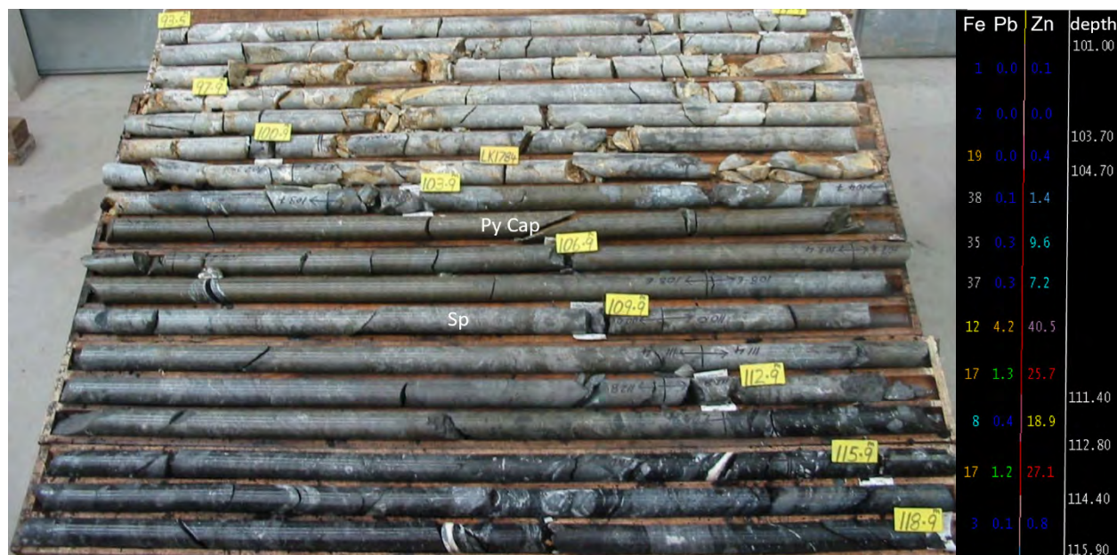
Figure 19: A typical interval through ore in the structural hanging-wall proximal to ore-controlling faults. Pyritic, black matrix breccias pass quickly into massive pyrite. This is often barren of zinc, as in this case, and forms a ‘pyrite cap’ above the economic ore. Zinc grades typically increase towards the bottom, (grades in % to right). The footwall contact and the Ballysteen beneath is commonly tectonized. (LK-1784, Bog-Zone East, Lisheen, box length 1.5m).
