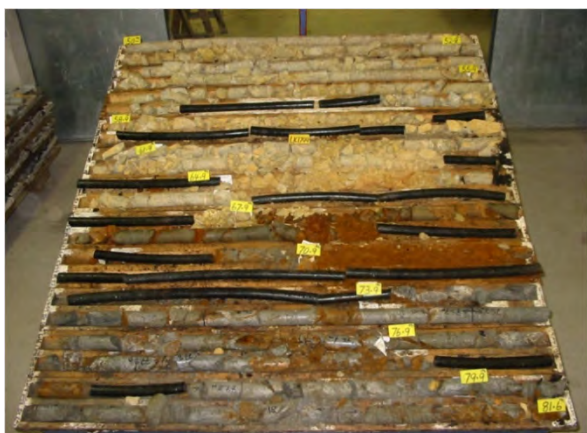
Figure 10: Pyritic ore is often extremely weathered adjacent to northwest-southeast structures and associated joints and locally causes considerable geotechnical challenges for mining. Sphalerite rich ore, as at the base of this image, is less susceptible.
