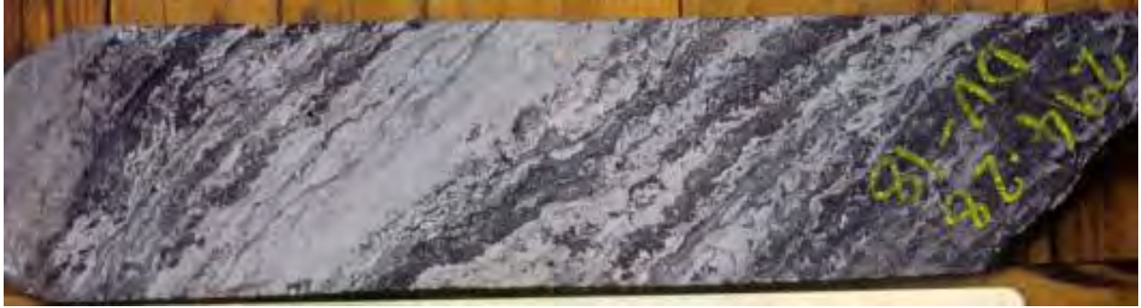
Figure 29 High-grade zinc mineralization at Duddar, Pakistan. Pale fine-grained sphalerite replaces algal or bacterial laminite in bedded carbonaceous limestone and mudstone. DU-18 284m, NQ core.
