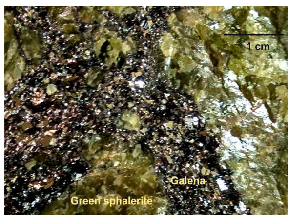
Figure 8: (Bottom Left) Pyrite (Py), Sphalerite (Sph) and galena (Gn) with extensive quartz veination, Zawarmala mine,
